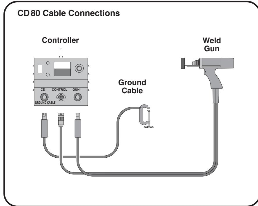
**NOTE:** All cables should be laid out straight or in large loops. Poor welds may result if welding cables are closely coiled or stacked up.
