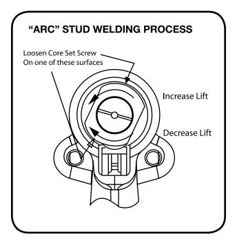
After properly setting the lift, retighten the nylon tipped set screw to keep the adjustable core in place. Replace the rear cap and tighten the rear cap screw. It is important that the rear cap is in place as the prevents dirt and other contaminants from entering the gun and fouling the lift mechanism.
