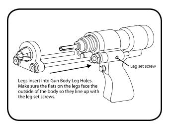
Insert the legs into the gun body leg retainers. Line up the flat on the leg with the set screw. The set screw will bite into the flat region and hold the leg securely. Tighten the set screws in the side of the legs. If the set screw bites into the round portion of the leg, it will damage the leg so it doesn't inset into the gun body leg retainer any more.
