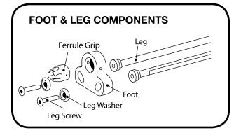
The foot is installed on the ends of the legs. Unscrew the flat head screws from the ends of the legs. Place the trim washers on the flat head screws and place the screws through the adjustment slots in the foot. Reattach the screws to the legs.
