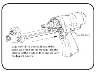
up the flat on the leg with the set screw. The set screw will bite into the flat region and hold the leg securely. Tighten the set screws in the side of the legs. If the set screw bites into the round portion of the leg, it will damage the leg so it doesn't inset into the gun body leg retainer any more.
