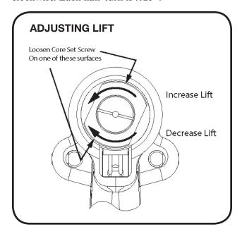
After properly setting the lift, retighten the nylon tipped set screw to keep the adjustable core in place. Replace the rear cap and tighten the rear cap screw. It is important that the rear cap is in place as this prevents dirt and other contaminants from entering the gun and fouling the lift mechanism.
