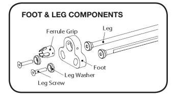
The foot is installed on the ends of the legs. Unscrew the flat head screws from the ends of the legs. Place the leg washers on the flat head screws and place the screws through the adjustment slots in the foot. Reattach the screws to the legs. Insert the legs into the gun body leg retainers. Line
