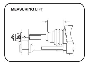
To measure gun lift, hold a scale against some fixed part of the tool. The front cover or the foot will work well. Press the trigger so the tool activates the lift mechanism. Now measure again. The lift is the difference between the two measurements.
